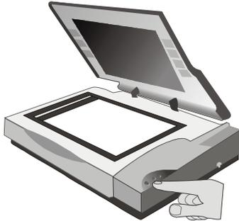
The LED power indicator on the front panel of the scanner lights up and flashes for about a minute and then remains lit, signifying that the scanner is ready.
